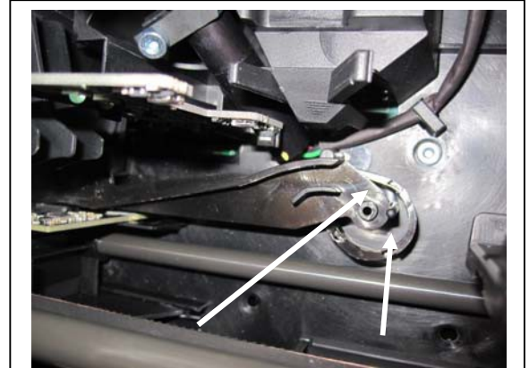
Correct spring position. The clip prevents the door from riding up.
